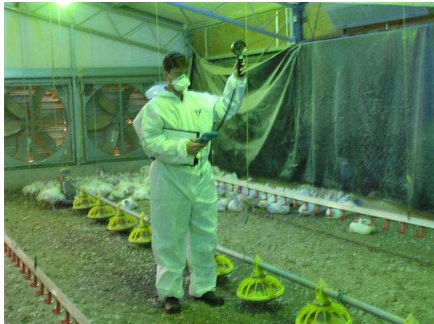
Chris using an anemometer to determine barn air flow rates. It's not all a holiday!
